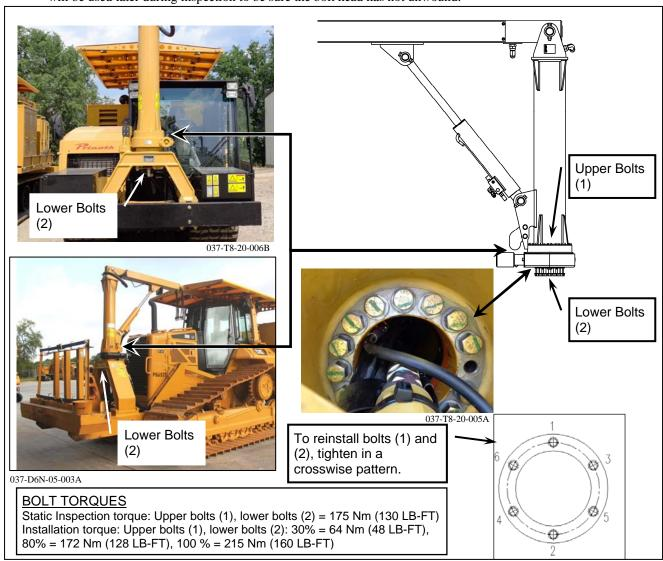
Figure 16: Slewing drive mounting bolts torque
