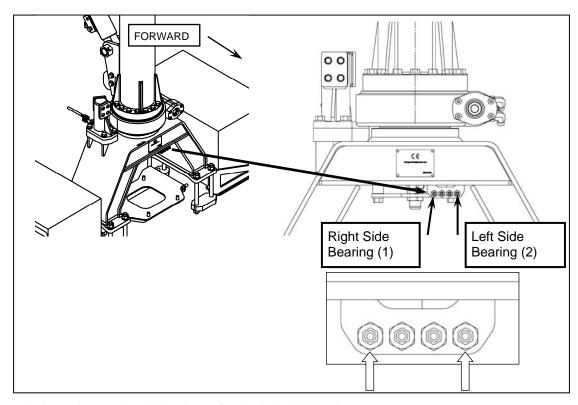
Figure 12: Slewing Drive Bearing lubrication Left and Right side location
