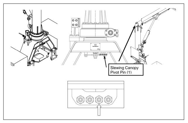
Figure 15: Slewing Canopy Pivot Pin lubrication location
