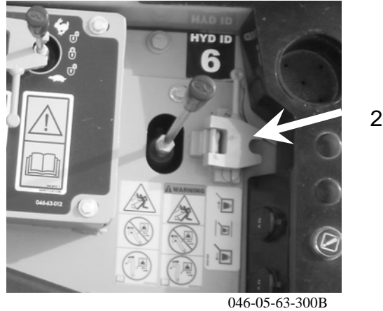
Figure 23: Counterweight control-lockout (2), open position
