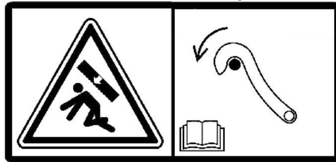
Figure 10: Counterweight crushing hazard, use lock lever (8)
