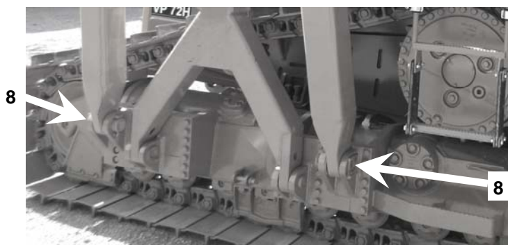
Figure 28: Location of pins for removal of boom
