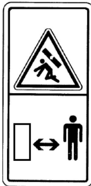
Figure 11: Counterweight crushing hazard and pinch point (9)
