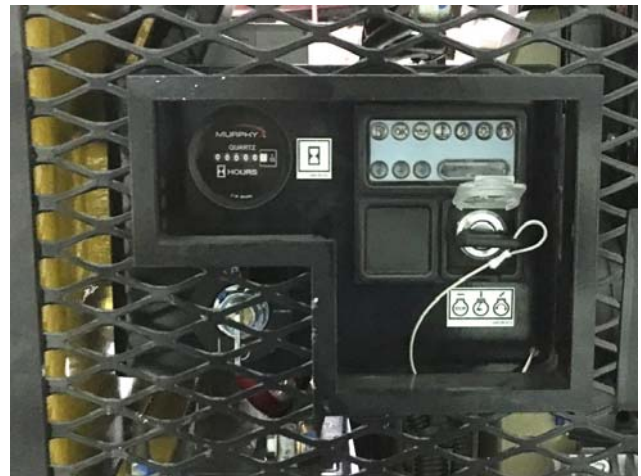
Operator control panel with doors closed. Lockout is accessible only with doors open for improved safety. 049-50-63-022B
