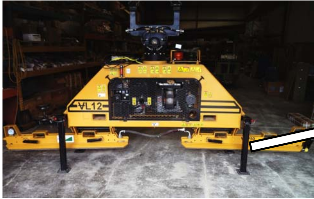
Tank stand legs in parked position for overnight storage.
