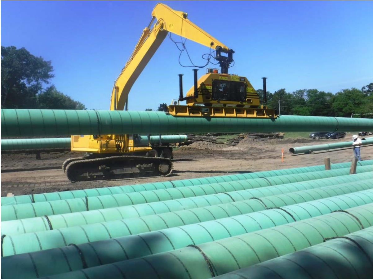
Large tank preserves vacuum level better when working repetitively and at high altitudes. 049-05-05-032B
