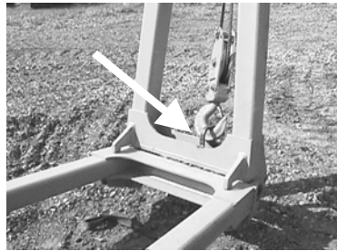
Figure 32: Hook block in folding boom stowing bracket.
