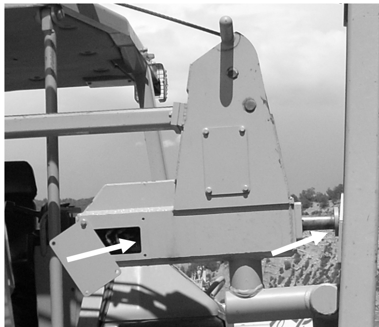
Figure 41: Check inner and outer boom stop bushings.
