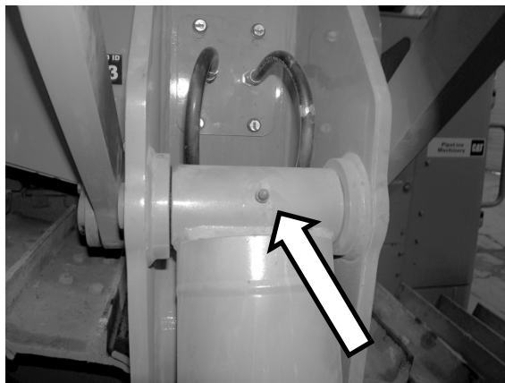
Figure 34: Counterweight cylinder bearings location
