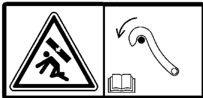
Figure 8: Counterweight crushing hazard, use lock lever (6)
