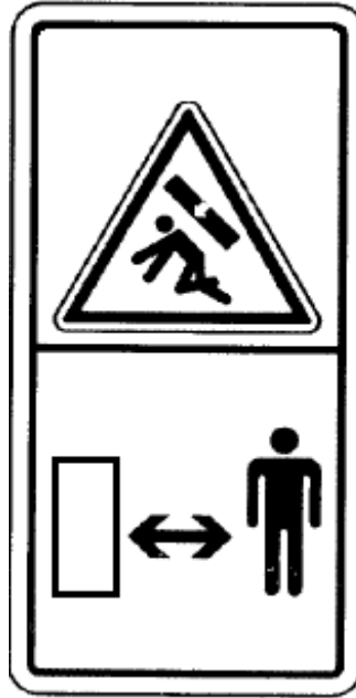
Figure 7: Counterweight crushing hazard and pinch point (5)
