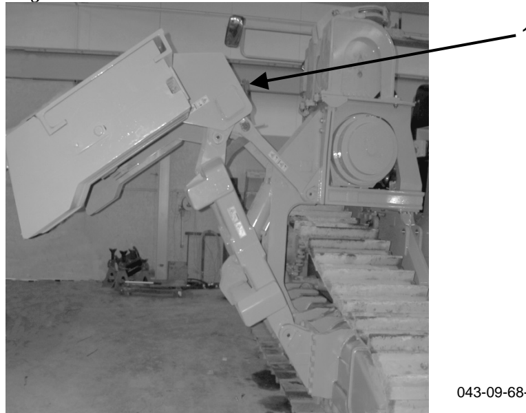
Figure 22: Counterweight Lock Lever (1) locked in the extended position, viewed from front
