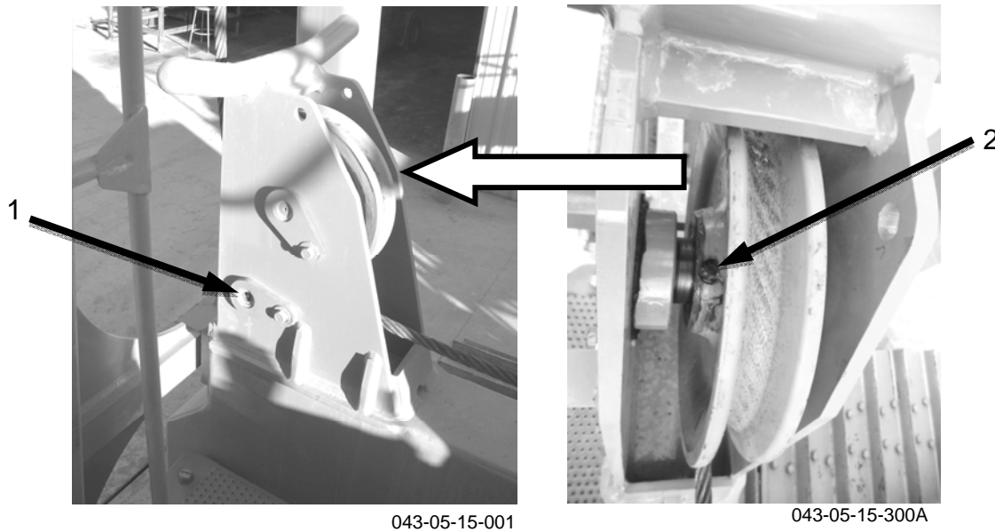
Figure 40: Fairlead sheave lubrication points
