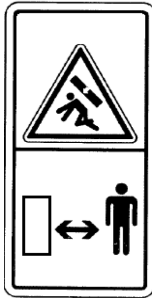
Figure 7: Counterweight crushing hazard and pinch point (5)
