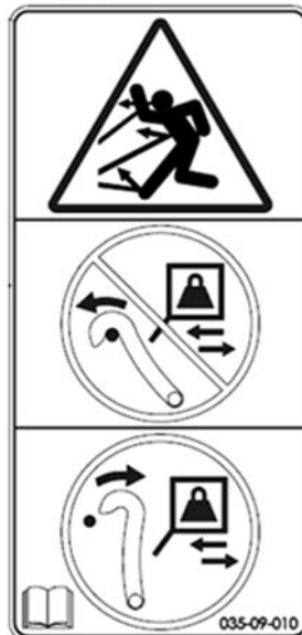
Figure 6: Thrown or flying objects - counterweight lock lever instruction (4)
