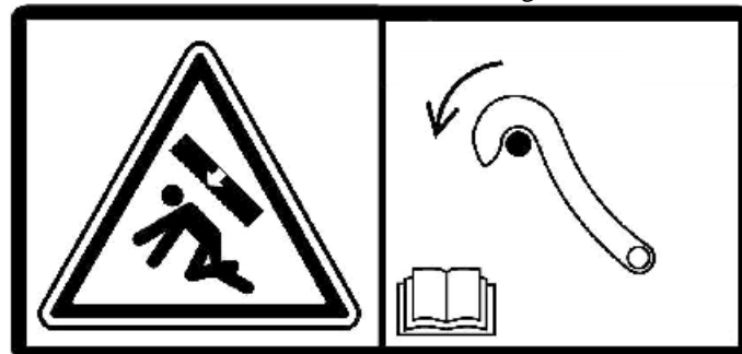
Figure 8: Counterweight crushing hazard, use lock lever (6)
