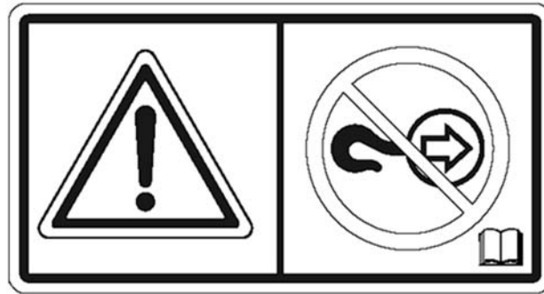
Figure 13: Equipment damage hazard, not a tow point (11)
