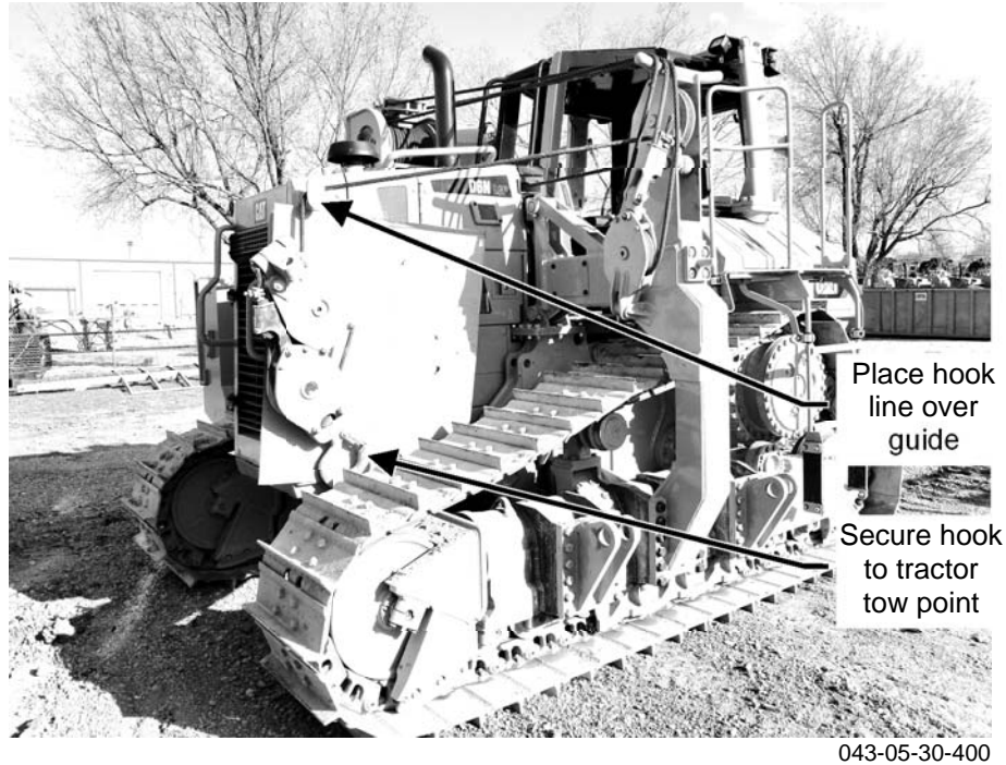
Figure 27: Secure Load and Hook Blocks for Transport
