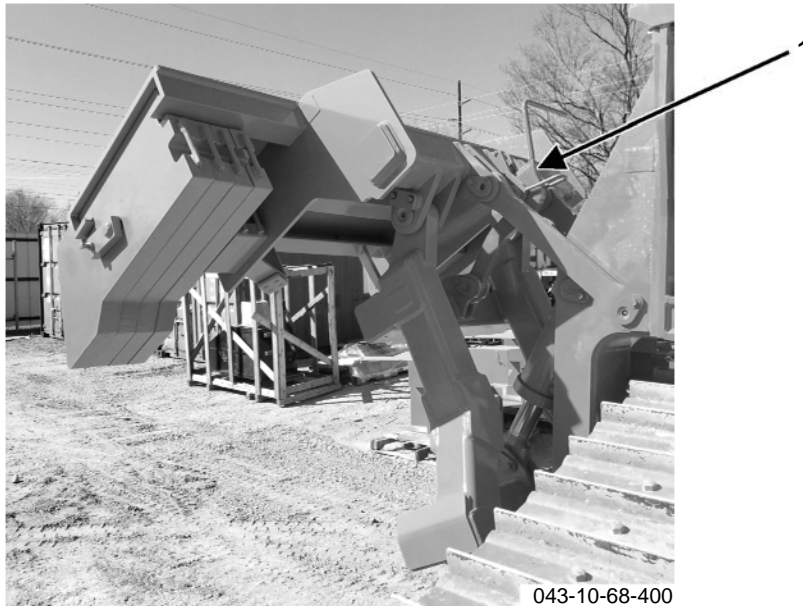
Figure 22: Counterweight Lock Lever (1) locked in the extended position, viewed from front
