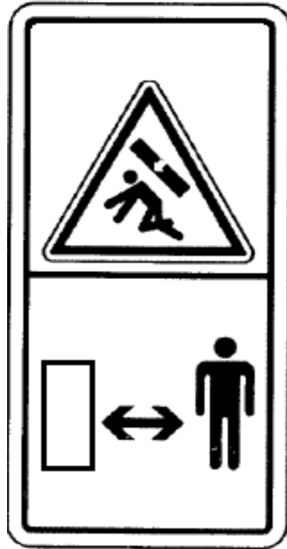
Figure 7: Counterweight crushing hazard and pinch point (5)
